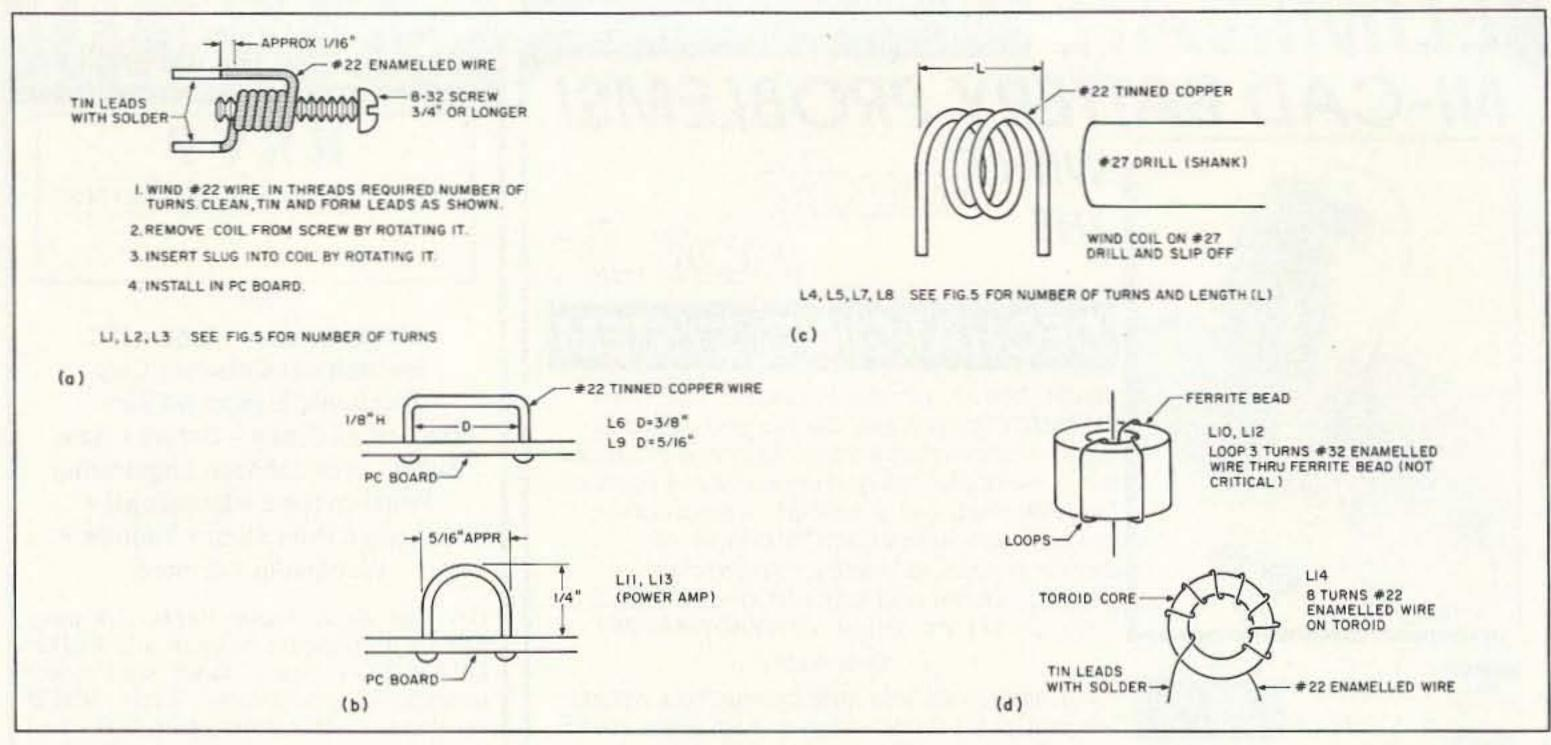
Figure 4. Coil construction.
